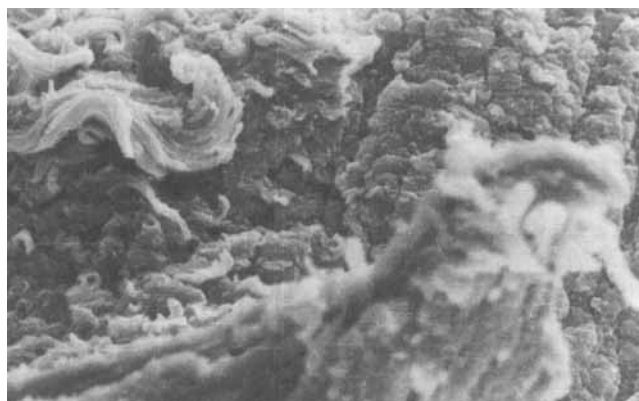
FIGURE 16 SEM fractogram of the blend B 7 (500×).
